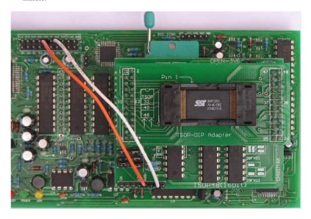
5. Connect two address jumper wire from board to programmer A19 and A20.
