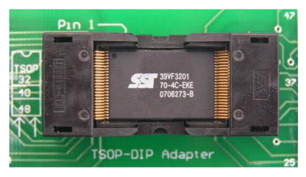
4. Place the adapter into the programmer ZIF and close the programmer ZIF socket handle.
